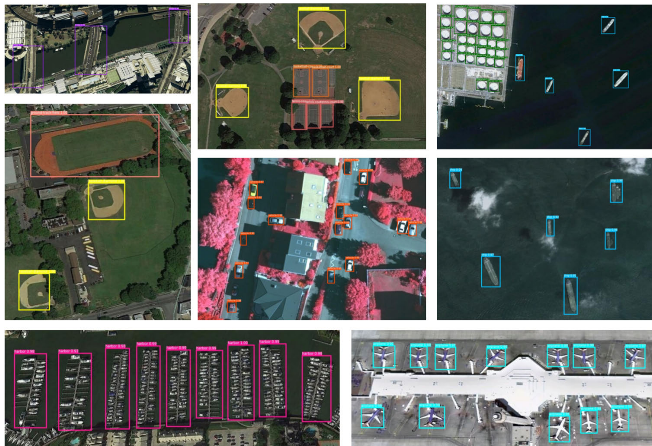
FIGURE 7. The detection results of PTAN on the NWPU VHR-10 dataset.
