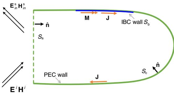
Fig. 1 Cavity with partial IBC wall is illuminated by plane wave
