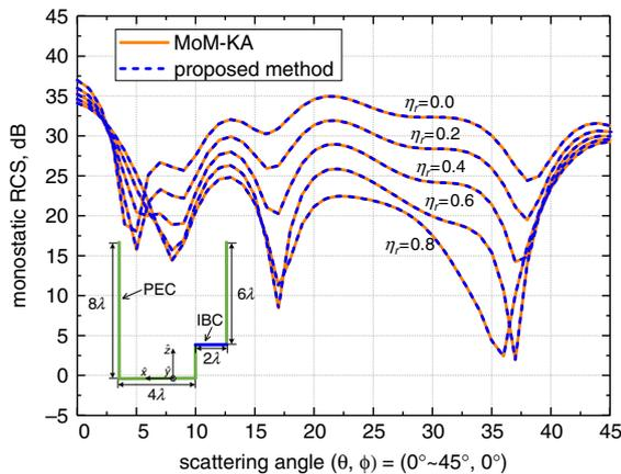
Fig. 3 Monostatic RCS of cavity with IBC wall and normalised surface impedance has different values
