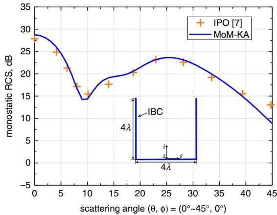
Fig. 2 Monostatic RCS of  $4\lambda \times 4\lambda$  IBC cylindrical cavity
